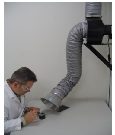
(Top) FE-1200 with a customized hood venting plasma cutting fumes. (Bottom) FE-500 shown at a soldering station.
